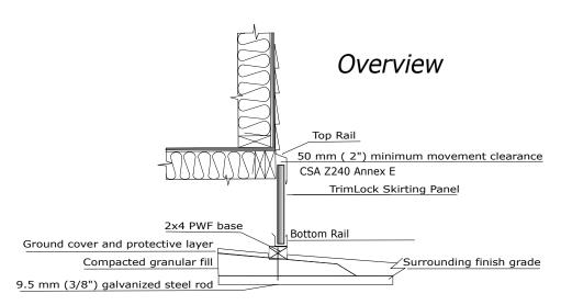
Note: Minimum movement clearance is to accommodate movement in areas susceptible to frost heave Wood in contact with ground should be PWF treated lumber
