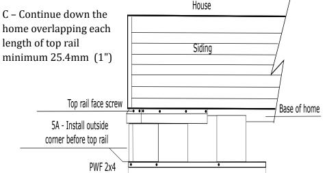
Note: In windy locations placement of each overlap should coincide with wind direction to reduce any possibility of any joint catching in the wind.
