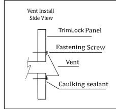
Cut a hole the size of the vent pipe through the skirting panel. Cut a wood back plate bigger then the vents' outside nailing flange and cut a center hole for the pipe. With the wood plate at the
